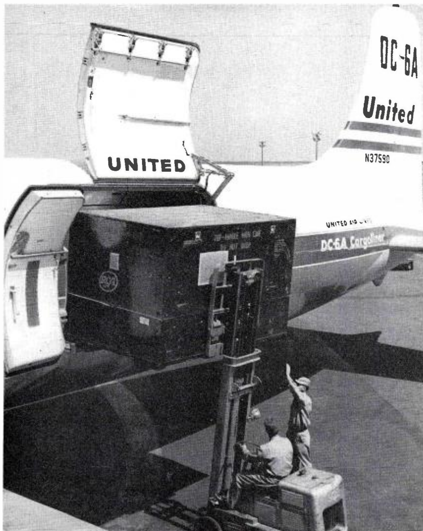
FIG. 1. Fast air shipments are made in emergencies. Here a transformer for a 50 kw transmitter is being loaded on a United Airlines cargo plane.
